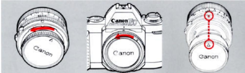
Turn the rear lens cap in the direction of the arrow until it stops. Then pull it off the lens.
