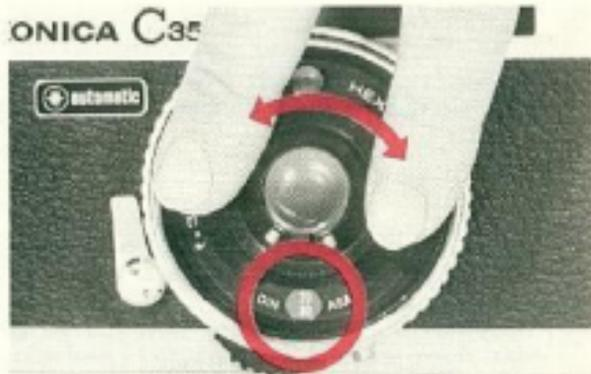
6. Turn the Film Speed Ring (9) and set your camera to the speed of the film you use in your camera. Note any intermediate point between film speed readings is unusable.
