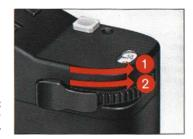
When the whole film is exposed, the transport lever no longer swings out fully and the release is blocked.
