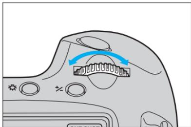
2 Turn the main dial to the left or right until the desired self-timer mode appears in the LCD panel.
