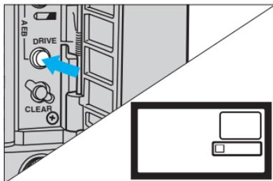
1 Open the palm door and press the film winding mode selector.
