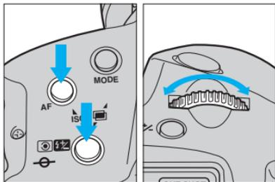
1 While simultaneously pressing the AF mode selector and metering mode selector/flash exposure compensation button, turn the main dial to the left or right until the desired film speed is displayed in the LCD panel.
