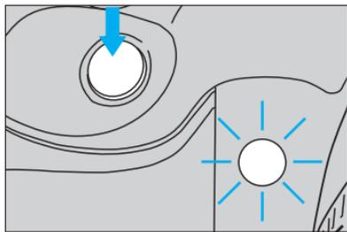
4 Press the shutter button completely. The self-timer lamp blinks to indicate that the self-timer function is operating. The lamp starts blinking faster two seconds before the picture is taken.
