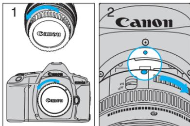
1 Remove the lens' rear dust cap and the camera's body cap by turning them counterclockwise.
