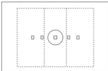
Operation of the built-in three-zone (center, right, left) automatic flash sensor corresponds to the five focusing points, increasing flash exposure precision by automatically weighting the exposure to the center when autofocusing at the center point, or to the left or right when autofocusing at one of the side points.
