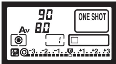
3 Releasing the metering mode selector / flash exposure compensation button completes the flash exposure compensation setting. The LCD panel returns to its normal condition and
