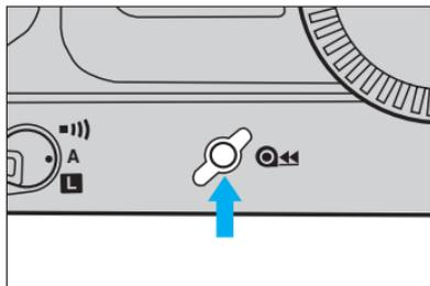
1 When rewinding starts, the film rewind indicator moves from right to left to show that the film is rewinding. At the same time, the LCD panel's frame counter counts down the number of frames.
