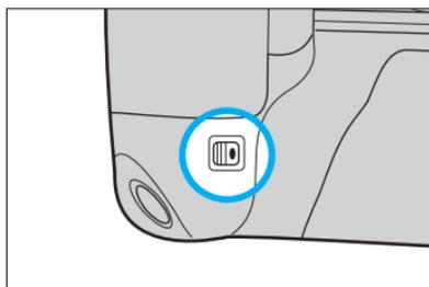
To use the vertical grip and the corresponding shutter button and AE lock button, turn on the ON/OFF switch.
